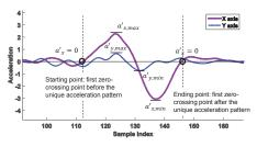
Figure 6: Searching for starting and ending points based on releasing and pressing points within an acceleration segment.
