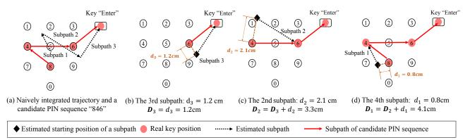
Figure 9: Example of point-wise Euclidean distance accumulation for candidate PIN sequence "846", where the real PIN is "419".
