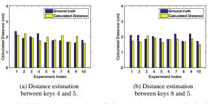
Figure 2: Distance estimation of the number pad on the Dell keyboard based on IMU.
