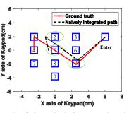
Figure 8: Example of the naively integrated trajectory having a large accumulated error cannot correctly map to the key positions of the PIN sequence "419" (though the estimation error of distance and direction of individual subpath is small).
