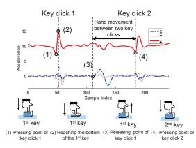
Figure 1: Acceleration patterns inherited from key entry activities, shown in the readings of a 3-axis accelerometer on IMU.
