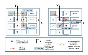
Figure 5: Illustration of the coordinate system on a typical key pad and examples of moving directions of key clicks, 13, 39, 16, and 68.
